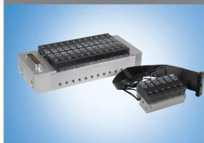
The compact, space-saving Series 554 3-way valves offer long life and high reliability. The direct-acting poppet valve has a flow rate of .022  $C_v$ . Rated for 12 and 24 VDC, the valves feature a green LED and optional quick-disconnect electrical connection. Manifold banks are available with a single row or double row of valves. The valve and manifolds can be purchased separately or as factory-assembled valve banks.
